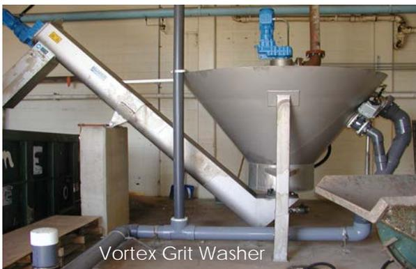
waste stream with the inflow/infiltration of rainwater and clear-water into the sanitary sewer system. The material removed is washed in a vortex grit washer, which removes any
